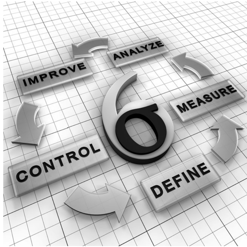
Figure 16.4 DMAIC, the Six Sigma cycle designed for improving existing processes.
