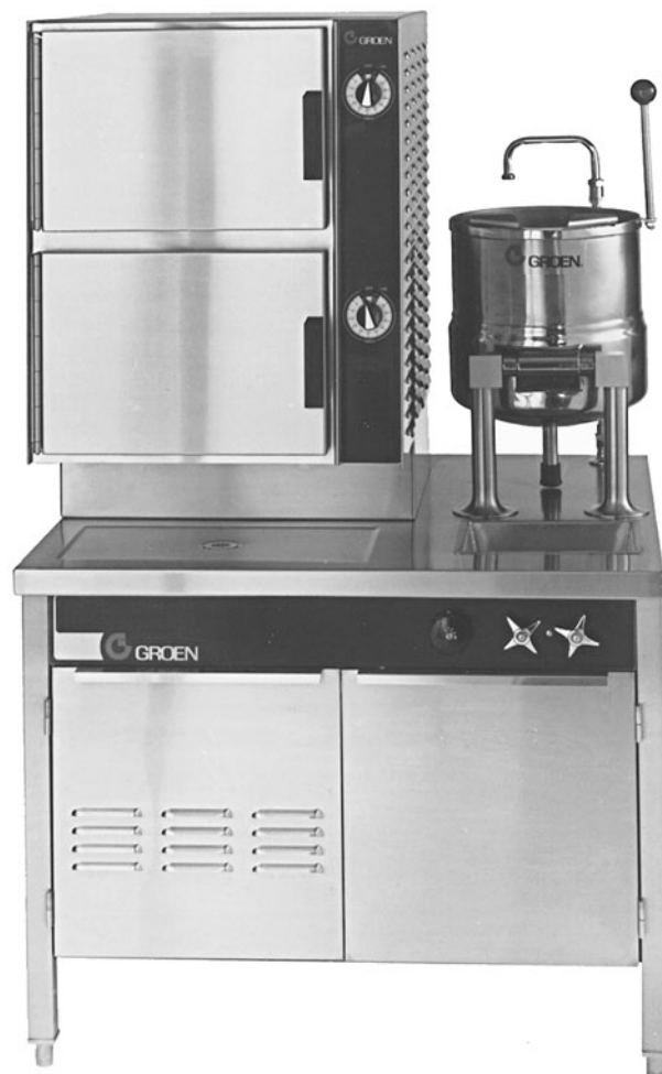
Figure B.34 Compartment pressureless steamers and jacketed kettle powered by a pressure boiler-in-base.
