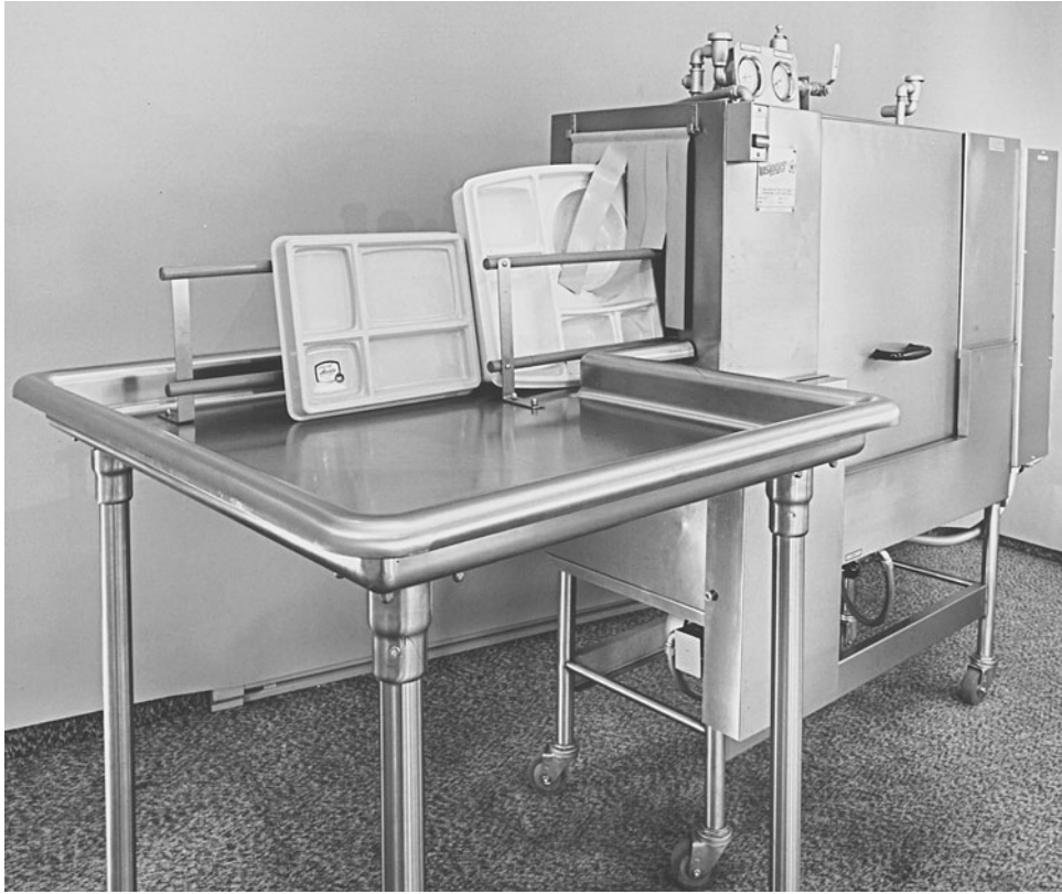
Figure B.48 Machine designed especially for washing trays.
