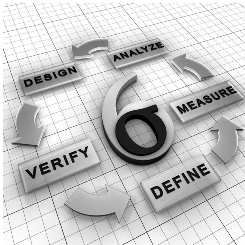
Figure 16.5 DMADV, the Six Sigma cycle designed for new products and processes.
