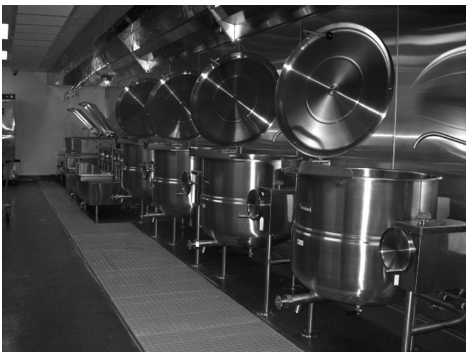
Figure 11.1 A bank of steam-jacketed kettles, steamers, and tilting braising pans in a large foodservice operation. Source: Robert Norlander, VP of Marketing, Cleveland Range, Cleveland, OH.
