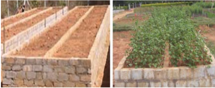
Figure 53.2 Specially constructed field root phenotyping structure to assess genetic variability in root traits in a large number of accessions [64].
