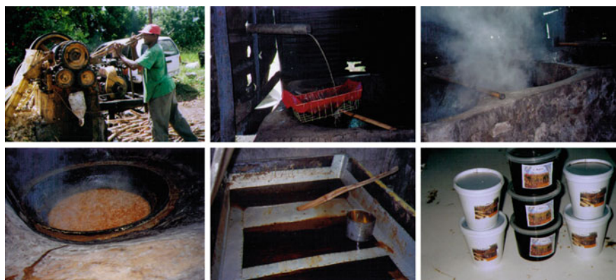
Fig. 1.2 Mr. Maye's Boiling House (2010) From top left : (1) the stalks of sugar cane are fed manually into the teeth of the crusher; (2) the resulting juice is funneled through a pvc pipe, and is strained into the first boiler; (3) steam from the three boilers can be seen. From bottom left : (4) the highly concentrated juice in the third cauldron; (5) syrup is allowed to cool in the trough while maintaining constant stirring; (6) the four styrofoam cups contain the solidified "head sugar". The three plastic cups contain "wet sugar" where the solid is dispersed in more molasses
