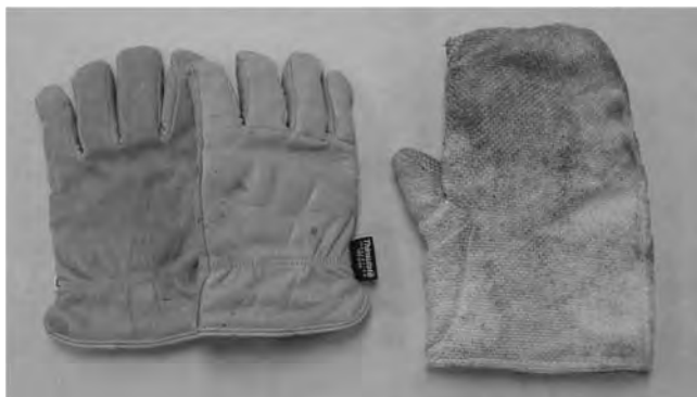
FIGURE 5.3.9.4 Insulated Gloves for Handling Cryogenics. The gloves on the left are best for holding cold objects since they will have better dexterity than the glove on the right (which can also be used for hot objects).
