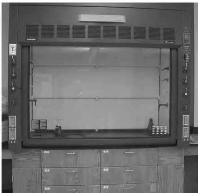
FIGURE 7.1.4.1 Laboratory Hood with a Vertical Sash. Sashes should always be closed except when arms and hands need to be accessing something inside the chemical hood. This both saves energy (for many modern hoods) and provides a shield against explosions and fires.
