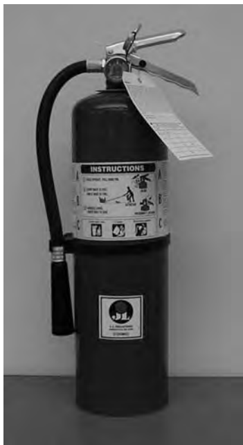
FIGURE 2.1.2.4 ABC Fire Extinguisher. This extinguisher can be used on Class A, B, and C fires. It is the most common type of extinguisher found in chemistry laboratories. It leaves a powdery mess after use, but this is better to clean up than the destruction a fire may cause.
