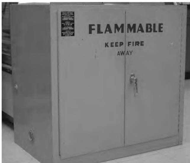
FIGURE 8.2.1.1 Flammables Storage Cabinet. Flammables liquids and solvents should be stored in the appropriate cabinet. Some cabinets are vented, some are not. This cabinet is not. To vent such a cabinet, the “bung hole” seen at the lower left is connected to a source of “make-up” air and a similar hole at the top of the right side of the cabinet is connected to piping to the exterior of the building. Simply opening these holes (without proper piping) would defeat the fire-rating capacity of the cabinet.
