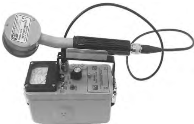
FIGURE 7.3.2.1 Ludlum Geiger–Müller Counter. These portable meters are routinely used to monitor an area for the presence of radioactive materials during and after handling these materials in laboratory operations. (Courtesy of Ludlum Measurements, Inc.)
