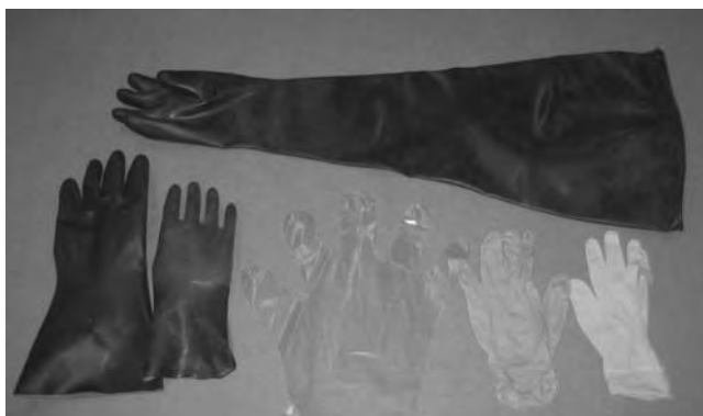
FIGURE 7.1.3.2 Various Types of Protective Gloves Used in Laboratories. Many styles of gloves, made with many different kinds of materials, are available. It is important to select the right glove to protect against the particular hazard. Degree of protection and dexterity vary considerably. There is no “universal” glove.
