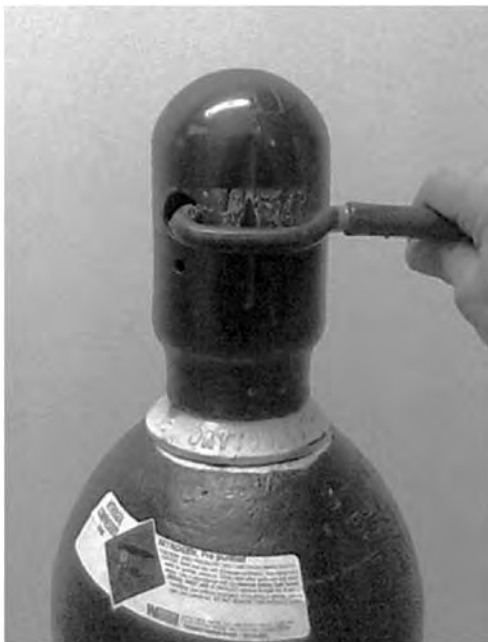
FIGURE 5.3.1.4 Tool to Remove Cylinder Cap. Do not try to force a stuck cylinder cap with a long screwdriver or other tool that goes through the cap. This may inadvertently open the tank by moving the main tank valve.
