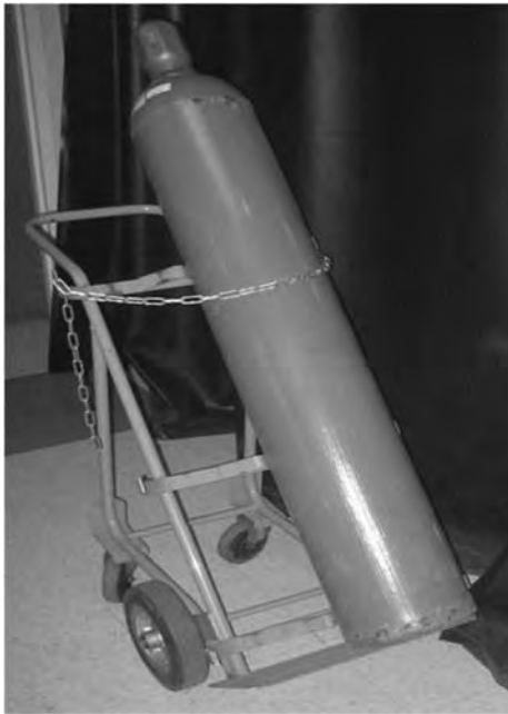
FIGURE 5.3.1.5 Cylinder Secured on Gas Cylinder Cart. Gas cylinders must always be moved on a cart, and the cylinder must be secured to the cart.
