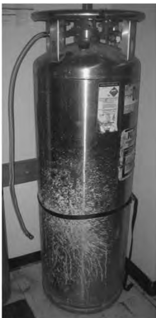
FIGURE 5.3.9.2 Large Commercial Dewar Tank. This tank holds about 180 L of liquid nitrogen. It is possible to withdraw the liquid directly from this tank and transfer the liquid to a smaller Dewar flask using the tube at the left in the picture.
