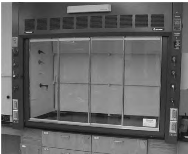
FIGURE 7.1.4.2 Laboratory Hood with Horizontal Sashes. These hoods are less frequently used but can offer similar protection as the vertical sash as long as they are not removed and the openings are kept to minimum size during operations and use.
