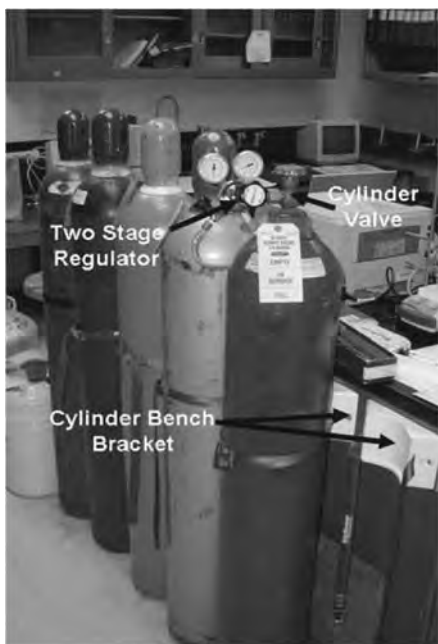
FIGURE 5.3.1.1 Gas Cylinders Showing Safety Brackets, Valves, and Regulators. Gas cylinders must always be secured to a laboratory bench or other immobile object so that they cannot fall over, snap off the regulator, and turn into missiles.
