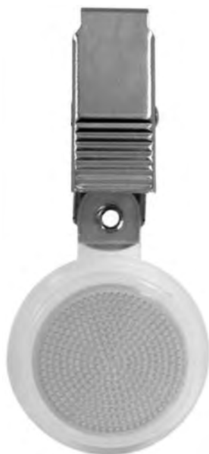
FIGURE 6.3.1.3 Passive Sampling Badge. The passive sampling badge contains a sorbent or a filter coated with a specific reactant that traps the contaminant(s) in the air. Passive monitors work by diffusion of the contaminant from the surrounding environment into the sorbent and the determination of the average air concentration is determined by validation testing. (Courtesy of SKC, Inc., Eighty Four, PA.)
