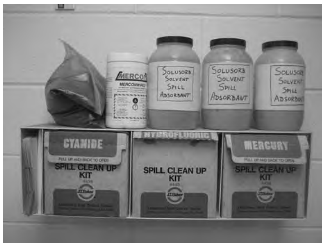
FIGURE 2.2.2.1 Chemical Spill Kit. There are many kinds of spill kits. It is best to know their location in laboratories since some spills should be contained as quickly as possible.
