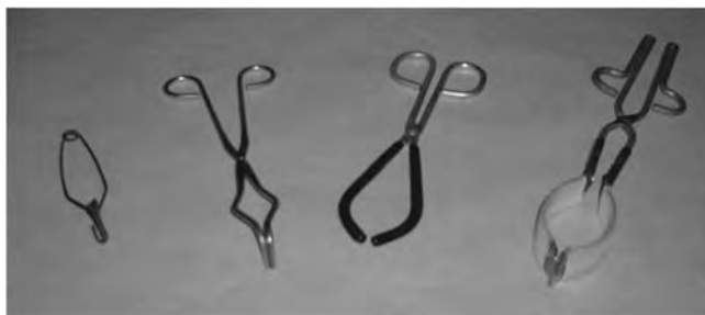
FIGURE 7.1.3.4 Tongs and Forceps Used in Laboratories. Use the right tool for the job. The beaker tongs with the rubber coatings are good for hot beakers but should not be used for really hot crucibles since this will melt the rubber.
