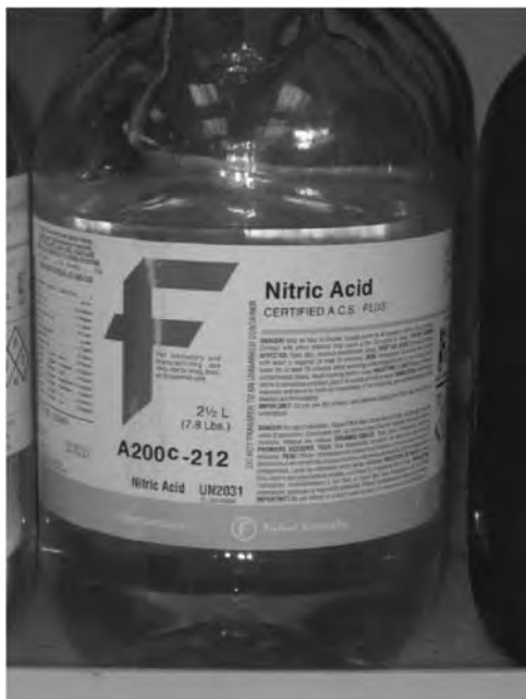
FIGURE 5.1.1.2 Concentrated Nitric Acid. Concentrated nitric acid is 15.8 M and 70% nitric acid by weight. It is very corrosive and produces toxic vapors. Exercise extreme caution if using this reagent.
