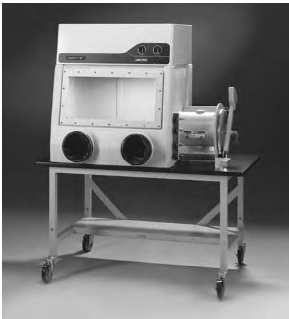
FIGURE 7.2.3.5 Glovebox. Gloveboxes are usually used in chemistry laboratories more for the protection of chemicals than lab personnel. Chemicals that are air- and/or water-sensitive can be used in these closed environments. This picture does not show a tank of nitrogen or argon that would usually be used for the interior atmosphere or various pumps and recirculating systems. The antechamber on the right is used to transfer materials in and out of the glovebox without allowing the laboratory atmosphere to enter the interior of the glovebox. (Courtesy of Labconco, Inc., Kansas City, MO.)
