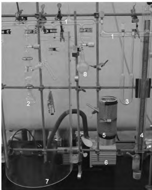
FIGURE 5.3.4.2 Laboratory Vacuum System. Low-pressure systems can have many configurations and components. This system shows a (1) manifold, (2) reaction flask, (3) trap, (4) manometer, (5) Dewar flask, (6) vacuum pump, (7) safety shield, and (8) storage bulb. (Photo courtesy of T. Leon Venable, Agnes Scott College, Decatur, Georgia.)
