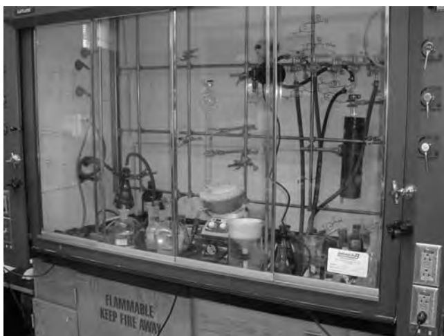
FIGURE 5.3.6.3 Cluttered Lab Hood. Lab hoods are well-known sources of clutter. Unused flasks, bottle beakers, and other lab ware are often left behind from previous experiments so that the user has to move things about to make room for his/her new work. What will you do if you were in a hurry and did not want to take time to clean this up?
