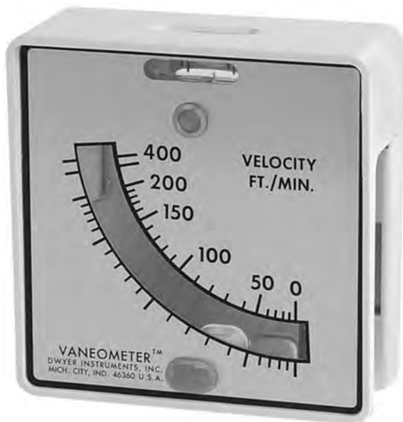
FIGURE 7.2.3.4 Vaneometer™ Used for Measuring Airflow in Laboratory Hood. These inexpensive devices can give a reasonable indication of airflow under a particular set of circumstances. (Courtesy of Dwyer Instruments, Inc., Michigan City, IN.)
