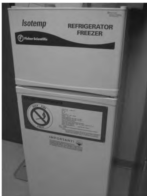
FIGURE 7.3.1.1 Explosion-Proof Refrigerator for Laboratories. These refrigerators are usually hard-wired into electrical supplies (so that they cannot accidentally become unplugged) and they have spark-proof interiors (internal switches and lights have been removed.)
