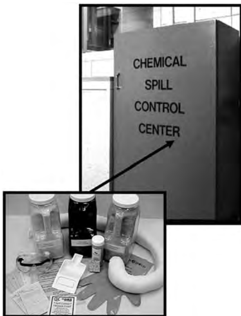
FIGURE 2.2.2.2 Chemical Spill Cabinet. Spill cabinets will contain useful equipment to handle many kinds of spills. The picture shows a “sock” that can be used to surround, contain, and absorb a spill.
