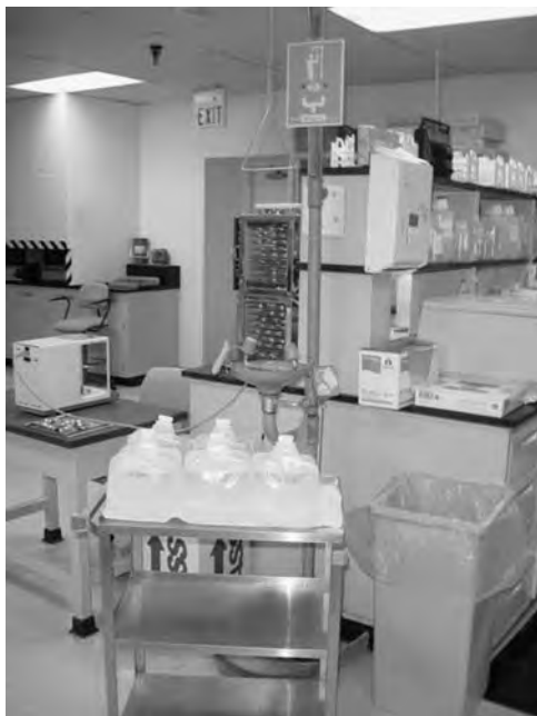
FIGURE 5.3.6.6 Cluttered Laboratory. In addition to the carts blocking the safety eyewash and safety shower, there are several other unsafe conditions in this laboratory. Can you spot them? (Courtesy of Harry J. Elston, Ph.D., CIH, Midwest Chemical Safety LLC, Buffalo, IL.)
