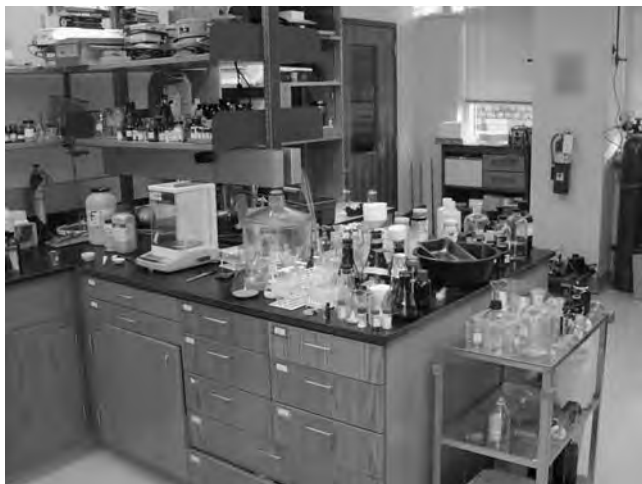
FIGURE 5.3.6.4 Cluttered Laboratory. Clearly, there are many bottles, vials, and containers at the edge waiting to be easily bumped onto the floor. There are other hazards in this lab. Can you spot them?
