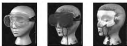
FIGURE 7.1.2.1 Degrees of Eye Protection from Simulated Splashes Using Varied Types of Eye Protection. The mannequin faces on the right show how effective each type of eye protection is against a chemical splash. Only the chemical splash goggles provide adequate protection and are the only acceptable form of eye protection in chemistry laboratories. (Courtesy of Linda Stroud, Ph.D., Science & Safety Consulting Services. Copyright © 2008 Science & Safety Consulting Services, Inc., Raleigh, NC.)
