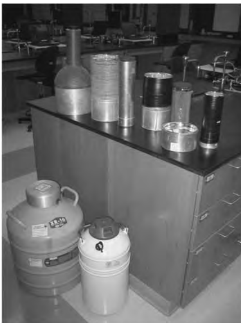
FIGURE 5.3.9.1 Assorted Dewar Flasks. Dewar flasks come in a variety of shapes and sizes.
