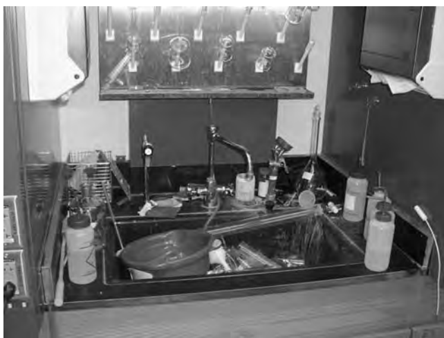
FIGURE 5.3.6.2 Cluttered Lab Sink. This sink is so cluttered with glassware that just trying to move something might result in breakage, and broken glass under water is hard to see. There might be odors coming from the sink. Obviously, the sink cannot be easily used without removing what is already in the sink.
