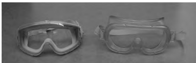
FIGURE 7.1.2.3 Chemical Splash Goggles. These goggles provide excellent splash protection and are relatively comfortable to wear, if sized properly.
