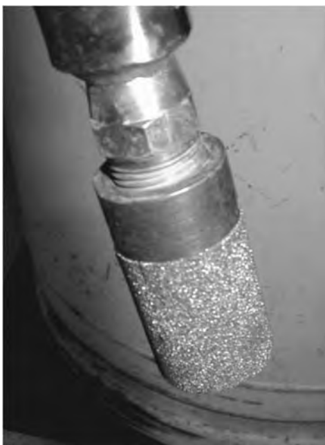
FIGURE 5.3.9.3 Phase Separator. This device allows a cryogenic liquid to be transferred with minimal splashing. (Courtesy of Office of Environmental Health and Radiation Safety, University of Pennsylvania, Philadelphia, PA.)
