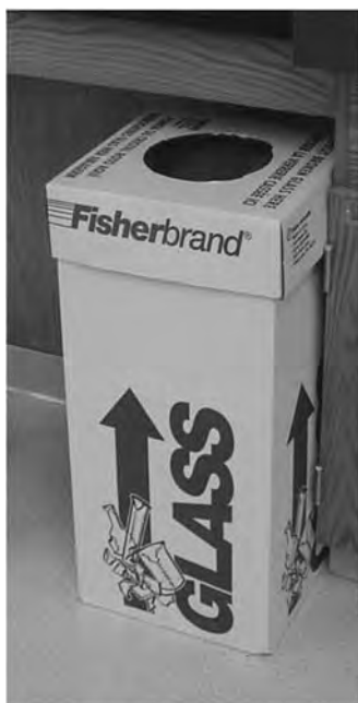
FIGURE 7.1.3.1 Broken Glass Container. Broken laboratory glass, if uncontaminated by chemical residues, should be placed in a container such as this.
