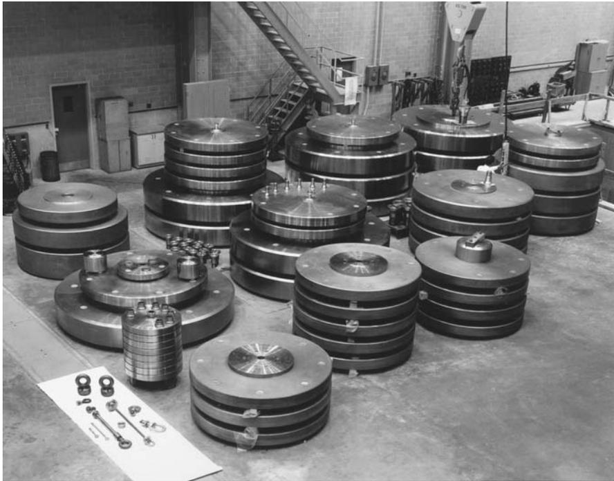
FIGURE 1.5 Large stainless steel weights that when assembled become a deadweight force machine.
